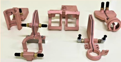
Examples of induction heating coils made with 3D printer
