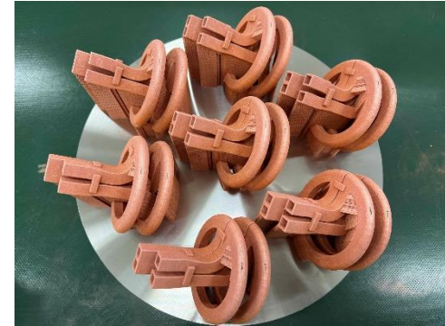
Example of induction heating coils made with 3D printer
