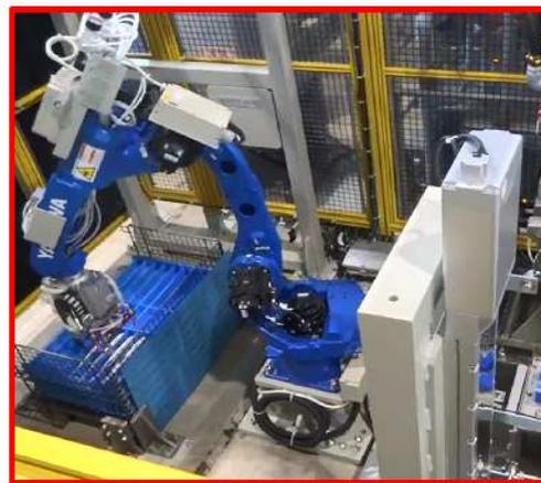
Realized full automation with latest 3D vision and industrial robots, from work removal to heat treatment, cleaning, inspection, and boxing
