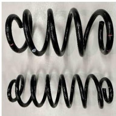
EV suspension spring using large-diameter ITW® (wire diameter: 17.2 mm)
