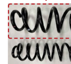
EV suspension spring using thick ITW® (wire diameter: 17.2mm)
